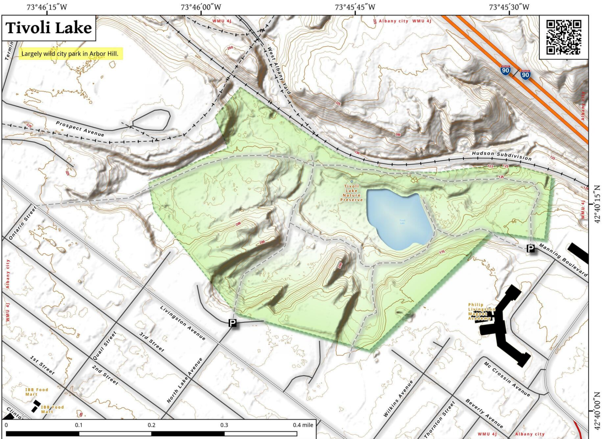
Tivoli Lake Map, April 3, 2016 by AndyArthur.org in QGIS 2.14.1-Essen and Python. Street Map is Copyright © OpenStreetMap contributors, CC BY-SA. NYSDEC Data: DEM, Borders, ADK Wetlands, Trails, Assets. True North. 1 inch = 0.1 miles. Projection: NAD83 / UTM zone 18N. Coordinates: 15" WGS 84. Contours are 5 feet using LIDAR.
